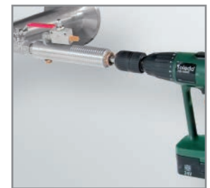
Drill under pressure with the CS Drill
