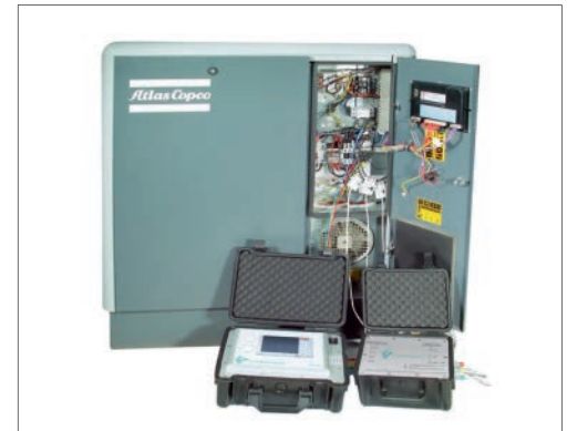
Example: Measurement at a compressor
